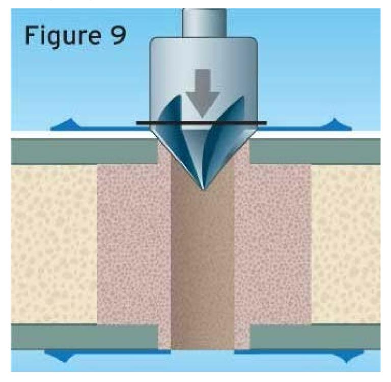
To give your bedding effort a better chance of long-term success, chamfer (bevel) the mounting holes with a countersink bit (Figure 9). This prevents squeezing out all of the sealant by over-tightening the fastener while compressing the sealant, creating a sort of O-ring. In addition, the thicker the sealant, the more it can stretch without rupturing, so the heavy band of sealant where the fastener passes through the deck will absorb more movement before failing.
