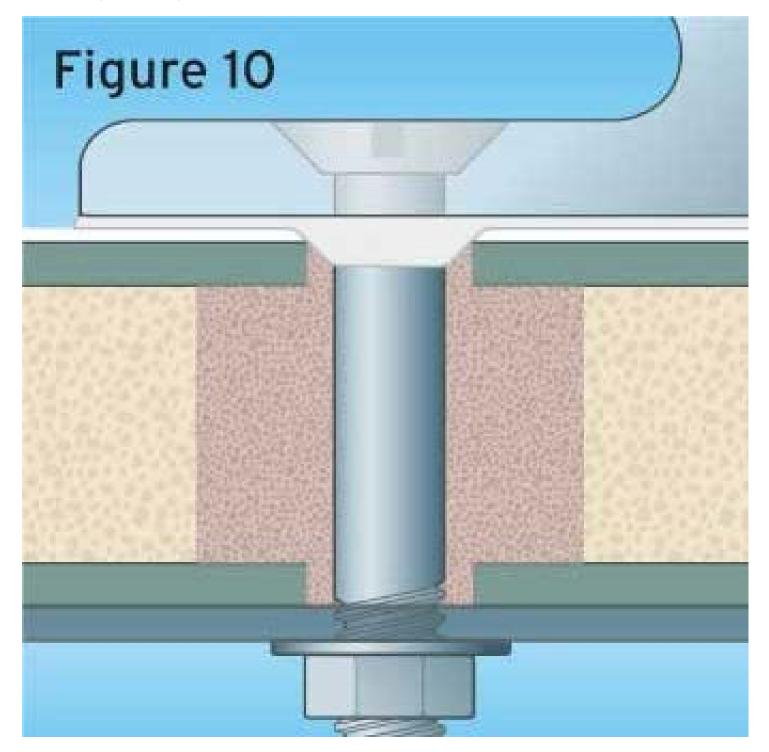
You can extend the life of the seal, particularly with silicone and, to a lesser degree, polysulfide by coming back after the sealant is fully cured and giving each of the nuts another half-turn. This reduces the amount the joint can flex and it puts the sealant under compression so that even if the bond fails, the clamped gasket will remain watertight. You must, however, take care not to turn the bolts, which will break their seal and do more harm than good.
